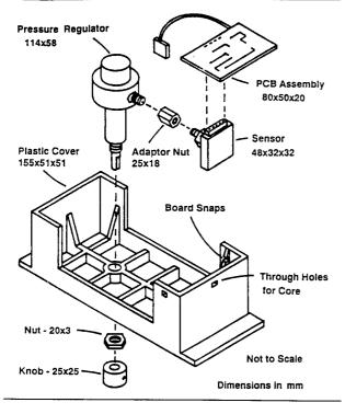
FIGURE 3: Proposed redesign for pressure recorder assembly [5]
