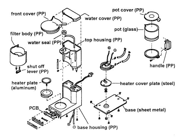
Figure 1 Exploded view of coffee maker
