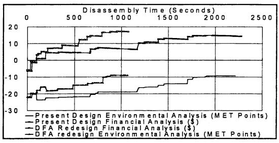
Figure 4 Disassembly analyses of an automatic washing machine
