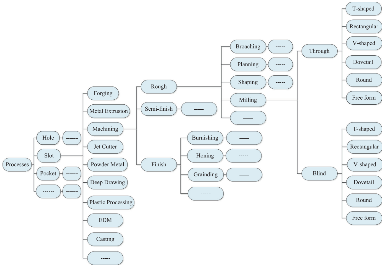
Fig. 2. Combined hierarchical manufacturing process and geometric classification of features.
