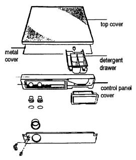
Figure 4. A washing machine subassembly.
