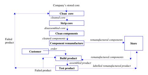
Fig. 1. A generic remanufacturing process chart.
