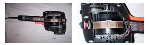
Fig. 5. Electric drill (repairable/reconditionable product) with detailed view of internal structure and motor.
