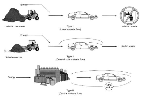
Fig. 5. Vehicle recycling models [47].
