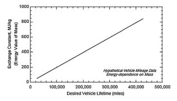
Fig. 11. Approximated relationship between vehicle mass and lifetime energy consumption, computed as a function of vehicle lifetime in miles [83].
