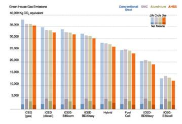
Fig. 13. Life cycle GHG's, varying by materials, power-trains and fuel sources [72].
