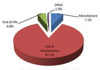
Fig. 8. Energy consumption in auto life cycle [1].
