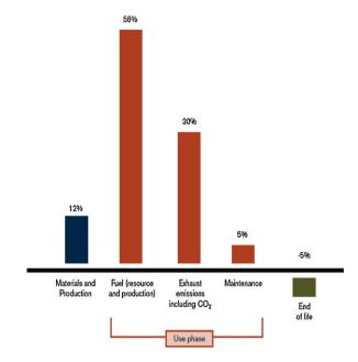
Fig. 14. Distribution of the environmental impact from a Volvo FH truck in long-haul operation [74].
