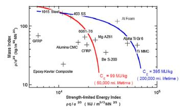
Fig. 12. The mass index plotted as a function of the energy index [83].
