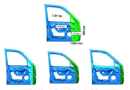
Fig. 6. Tailor welded blank applied for door inner [50].
