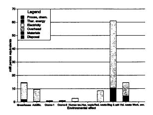
Figure 5 Environmental profile for a color TV set. Example of output from the EDIP-tool, reproduced (35).
