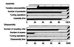
Figure 7. Applying the ABC method to an electric saw (68) Old design: white bars. New design: black bars.
