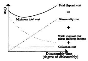
Figure 2 Total cost of disposal in a disassembly scenario (46).
