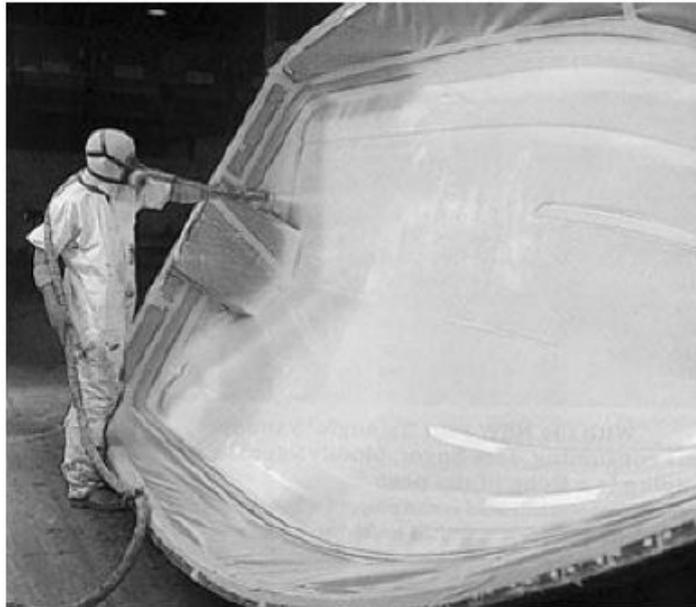
FIGURE 8.9 Spray-up technique. (Courtesy of Owens Corning. Used with permission.)
