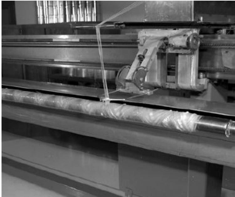
**FIGURE 8.20** Filament winding apparatus. (Courtesy of Owens Corning. Used with permission.)
